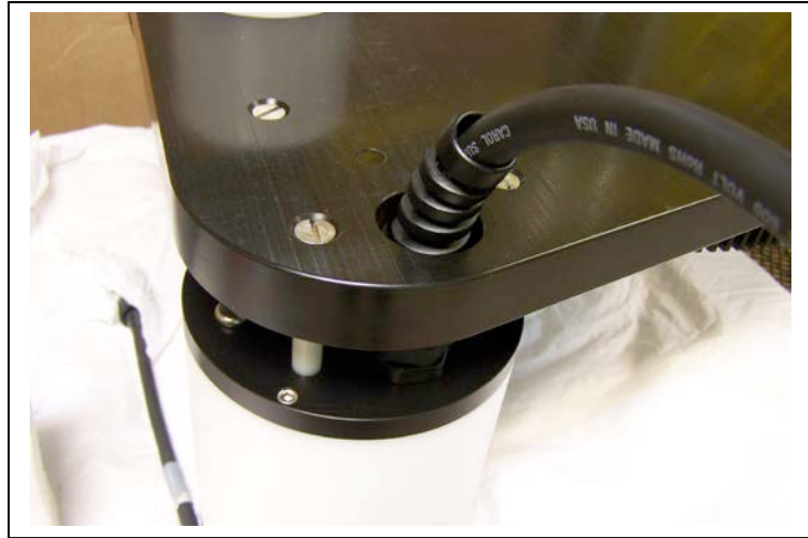
Figure I-5: Fit Motor Cable Down Through Hole in Rotator Plate
