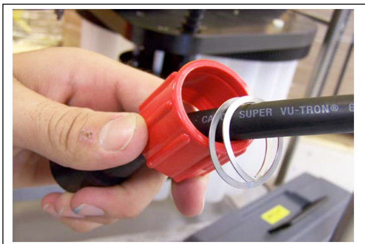
Figure I-4: Slide Locking Collar Off Motor Cable and Twist Off Locking Ring
