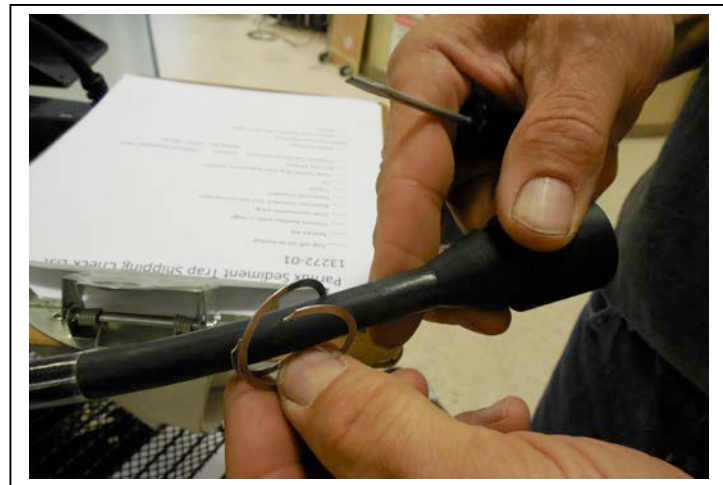
Figure I-4: Slide Locking Collar Off Motor Cable and Twist Off Locking Ring
