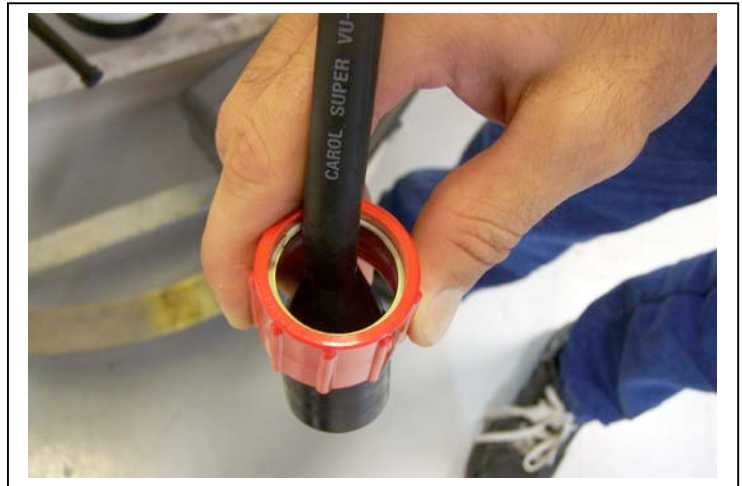
Figure I-2: Unscrew Locking Collar and Unplug Bulkhead Connector
