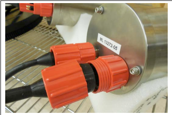
Figure I-2: Unscrew Locking Collar and Unplug Bulkhead Connector
